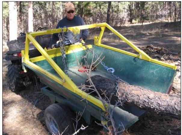
The winch cable is taken off, and the choker chain is set into a notch to keep the log from sliding back off the trailer while on the way to the landing.
