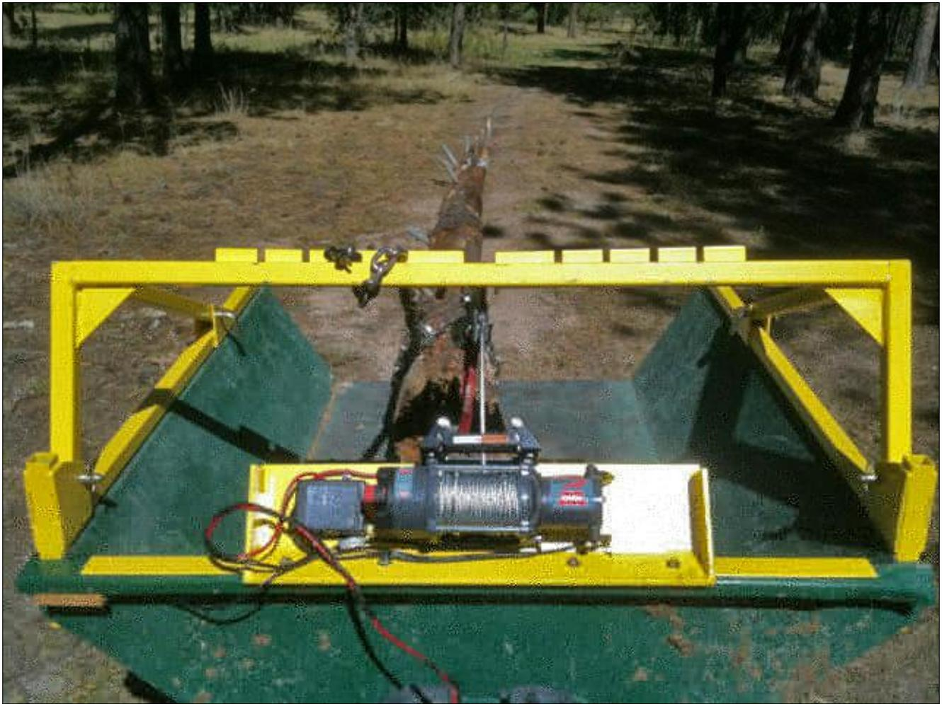
The upper cross-over bar carries the removable snatch block, which raises the winching point for a more advantageous angle of approach to the trailer bed. The notches allow the choker chains to be attached to the frame easily. This takes the stress off the winch and fairlead while moving the logs over stumps, rough ground and through brush.
