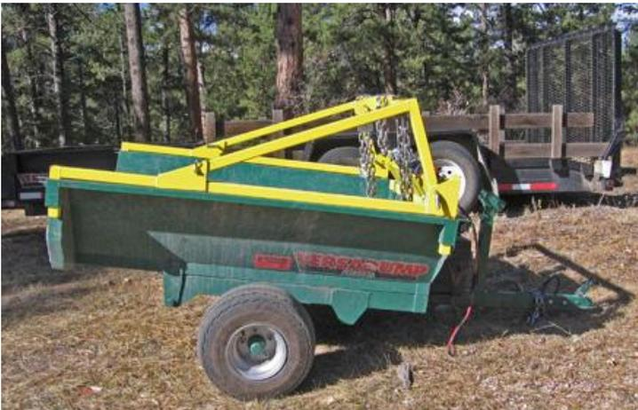
One woodland owner saw the potential to utilize his ATV and dump trailer to move logs efficiently, safely and with less soil and vegetation disturbance. What was missing was a way to get the front end of the log up into the trailer bed and hold them there during transport. The solution was to add a custom winching frame to the trailer.
