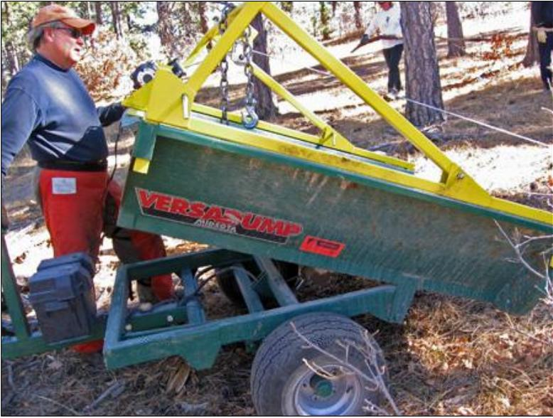
When the log is within about 10-12 feet and directly behind the trailer, the trailer bed is raised. This accomplishes two things; (1) It raises the angle of the winch line, and (2) it lowers the rear of the bed closer to the ground.
